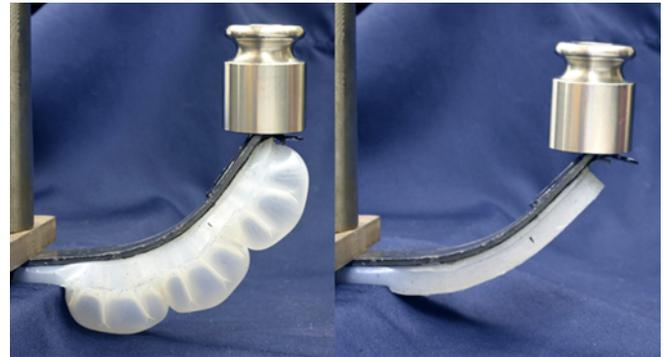
Fig. 1. Left: Softened variable stiffness pneumatic device inflated and supporting a 200g mass. Right: Supporting the same mass in a rigid material state with no power input. Weight is supported by a platform secured to the end of the finger.
