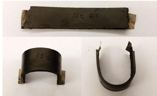
Fig. 2. Top: Variable stiffness sample in initial flat configuration. Bottom: Variable stiffness sample bent into a curve demonstrates passive holding of a deformed shape. The sample is approximately 10cm from end to end, not including the conductive fabric electrodes.
